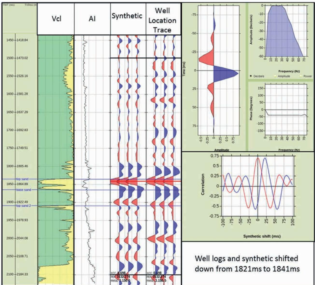
Figure 2 'Phase match' well tie at the well location using the Adaptive Technique. (Note colours for the correlogram are blue=pre-shift, red=post shift).
