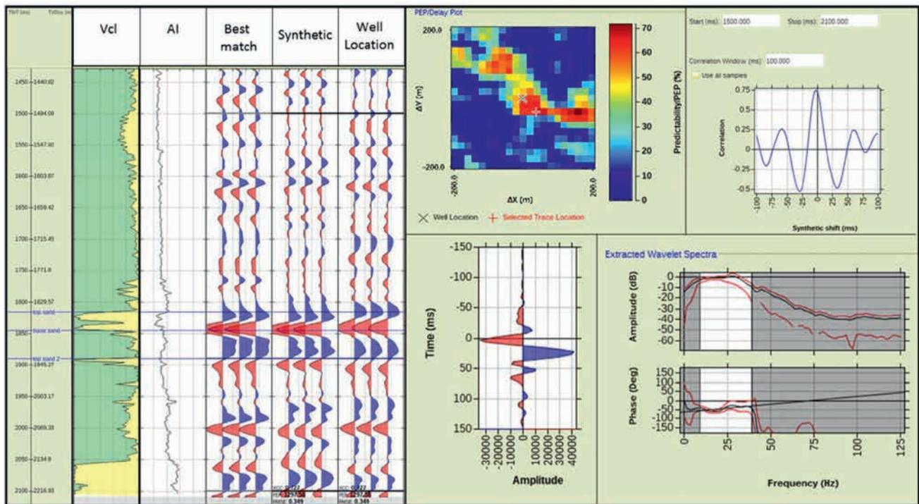
**Figure 1** Example of a ‘Phase Match’ Tie using White’s (1980) matching technique. The extracted wavelet is not symmetrical and has a phase intercept of about  $-60^\circ$  (see text for discussion). The wavelet lag has been added in the synthetic to illustrate the quality of the tie. Note that owing to the phase rotation and shift the marker horizons are not correctly referenced with respect to the seismic loops.
