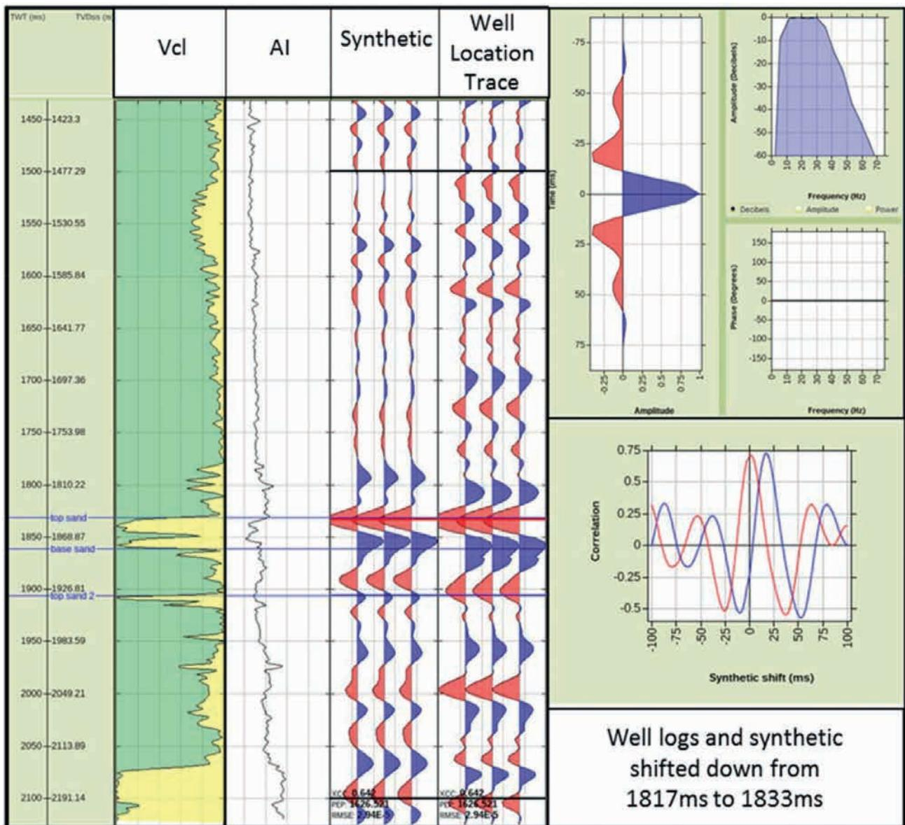
**Figure 3** Zero phase tie (with positive standard polarity wavelet) at the well location after phase rotation of +60°. The top and base of the low impedance sand now correlate clearly with a trough and peak respectively.
