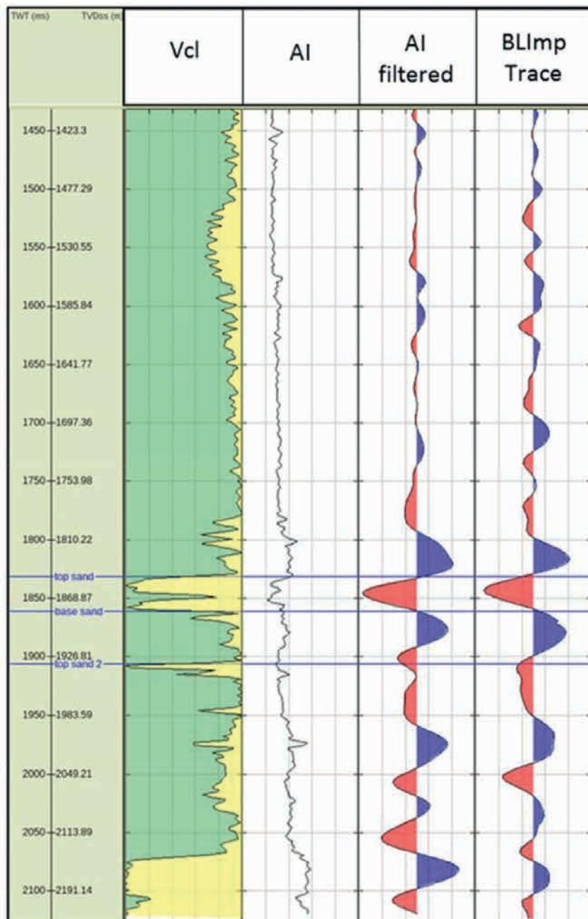
**Figure 4** Bandlimited impedance tie. The sand is evident as a low impedance layer (trough) with the top and base of the sand located close to the upper and lower zero crossing of the trough.
